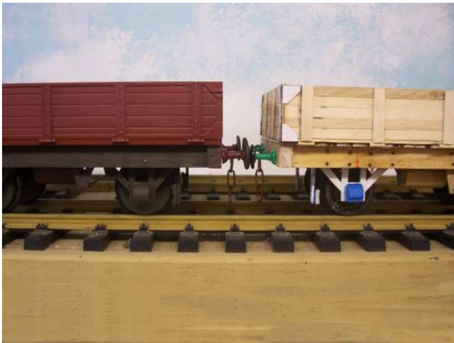
Sides have corner bracing cleats that double up as latch locations for the drop sides.
