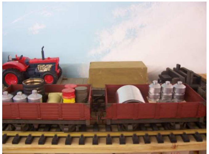
Sides have corner bracing cleats that double up as latch locations for the drop sides.
